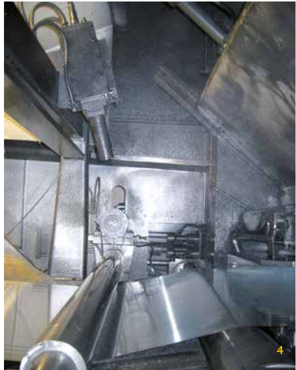
1 LSV with protection housings to measure casting speed and length in a billet caster
