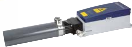
LSV-A-120 Air Wipe with quick exchange window A front-mounted, aerodynamically optimized air wipe unit keeps the sensor's optical window free of dust and steam. For cleaning or replacement, the quick release window can be easily exchanged.
