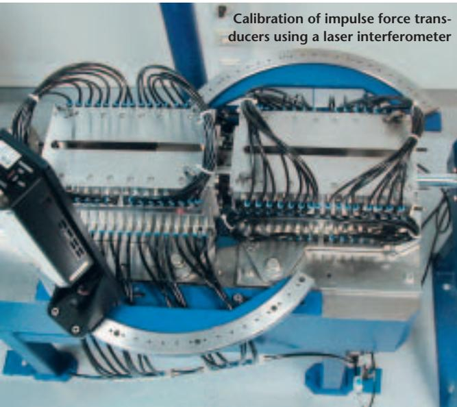
Calibration of impulse force transducers using a laser interferometer
