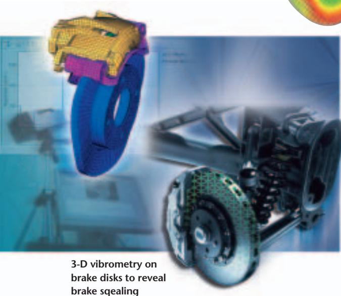
3-D vibrometry on brake disks to reveal brake squealing
