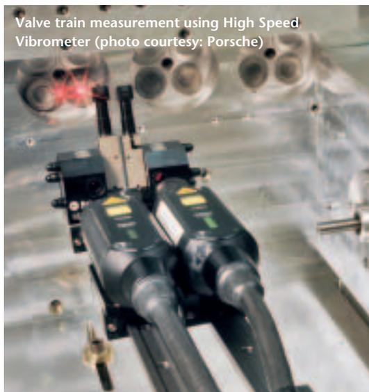
Valve train measurement using High Speed Vibrometer (photo courtesy: Porsche)
