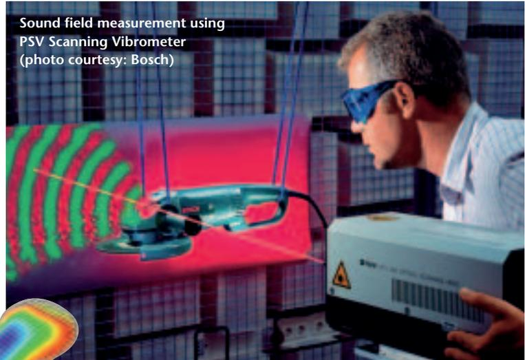
Sound field measurement using PSV Scanning Vibrometer (photo courtesy: Bosch)
