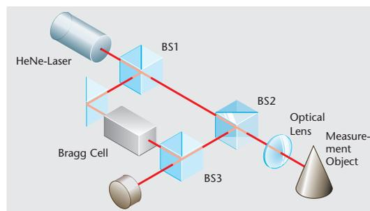
objects, delicate structures or ultrasonic devices are all made possible by non-contact laser vibrometry.
