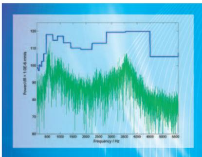
**Figure 5: Green: spectrum of a signal, blue: one-third octave band level of the spectrum**
