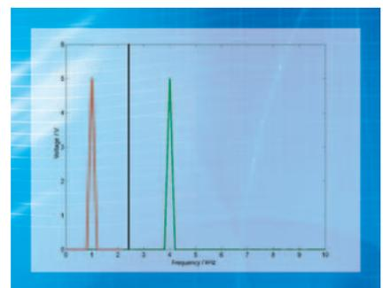
**Figure 4: Results of frequency analysis of both signals from fig. 3; green: real frequency, red: pseudo-frequency through Aliasing**
