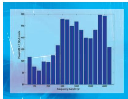
**Figure 6: One-third octave band level spectrum from fig. 5 (frequency axis is logarithmic)**
