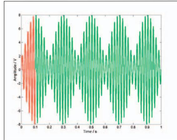
**Figure 1: The increased resolution of a long measurement versus a short measurement time; red: 0.1 s measurement duration; green: 1 s measurement duration**
