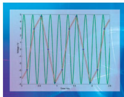
**Figure 3: Digitalization of a 4 kHz signal; green: sample frequency 10 kHz, red: sample frequency 5 kHz**
